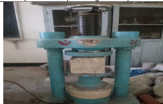
Fig4: During Compression Test of the Cubes
